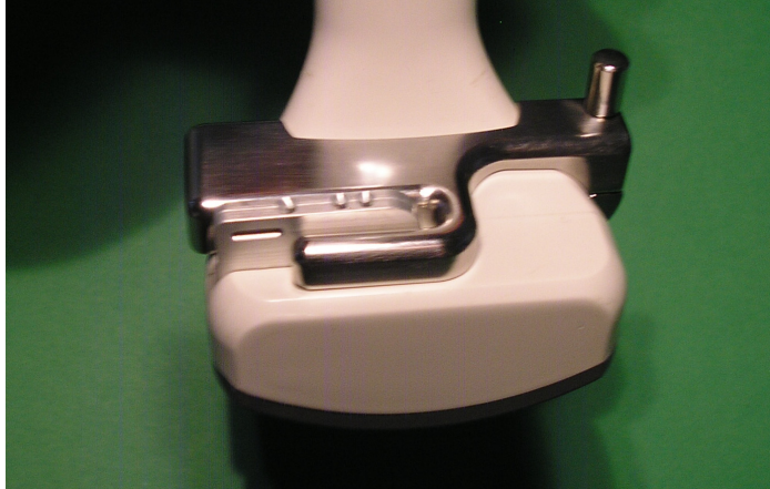
Fig. 13: Safety Catch Closed
